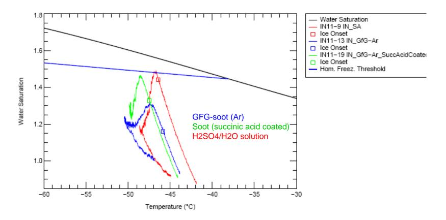
Coating of GfG-soot aerosol with succinic acid increases onset value of S<sub>ice</sub> for freezing markedly (same effect was found for sulphuric acid coating, published in Möhler et al, JGR 2005)
