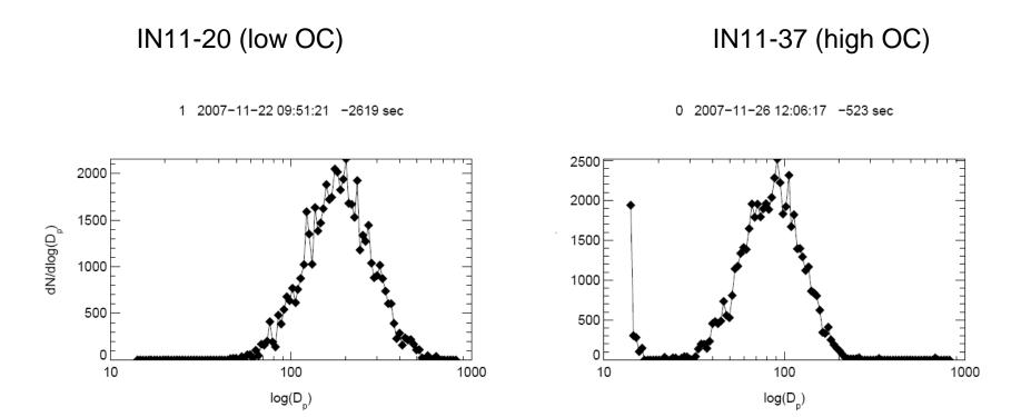
Möhler et al., 2005: "... increasing amount of OC condensing on the soot particles causes the initial aggregate structure to collapse to more compact particles with smaller mobility equivalent diameter ... "
