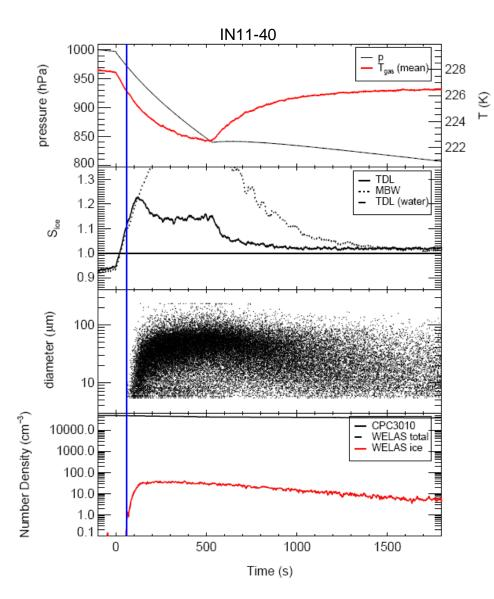
Synthetic air was passed over Oxalic Acid Dihydrate (heated up to 120°C in a glass tube) and injected into the cold AIDA (time period: 2h)
