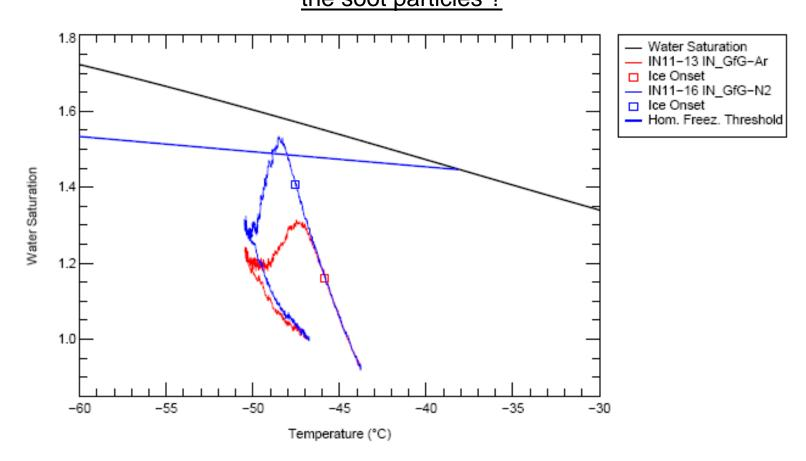
AIDA experiments are showing clearly the influence of the used carrier gas on IN properties of GfG-soot aerosol
