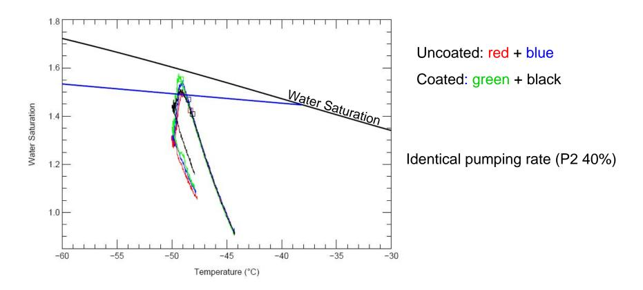
IN11-24: C = 1260 cm<sup>-3</sup>, ice active fraction: 0.5%, Ice onset: T = -49.1°C/S<sub>ice</sub> = 1.55 IN11-25: C = 910 cm<sup>-3</sup>, ice active fraction: 0.2%, Ice onset: T = -48.1°C/S<sub>ice</sub> = 1.40
