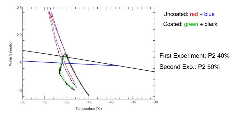
IN11-34: C = 1000 cm<sup>-3</sup>, ice active fraction: 0.6%, Ice onset: T = -50.0 °C/S<sub>ic e</sub>= 1.60 IN11-35: C = 720 cm<sup>-3</sup>, ice active fraction: 1.2%, Ice onset: T = -50.0 °C/S<sub>ice</sub> = 1.62
