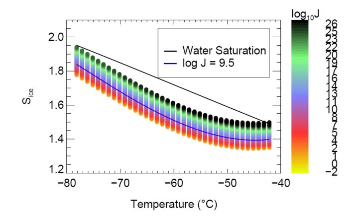
2d polynomial fit to surface provides parameterisation for J with  $J=J(T,S_{ice})$  suitable for proving with process model MAID
