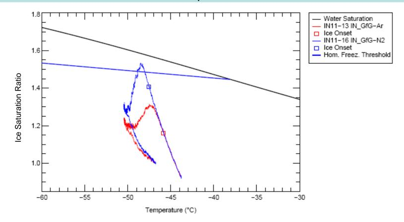
AIDA experiments are showing clearly the influence of the used carrier gas on IN properties of GfG-soot aerosol
